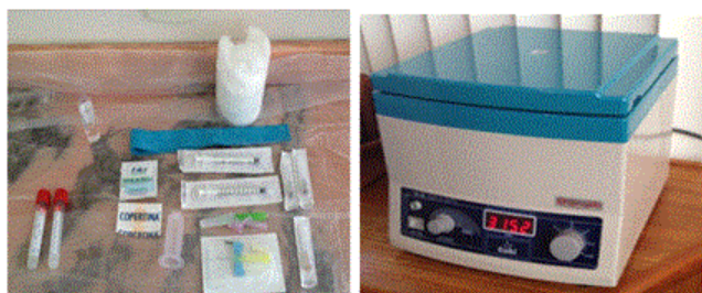
Figure 2: Syringes to be used and Centrifuge used for separation of blood cells.
