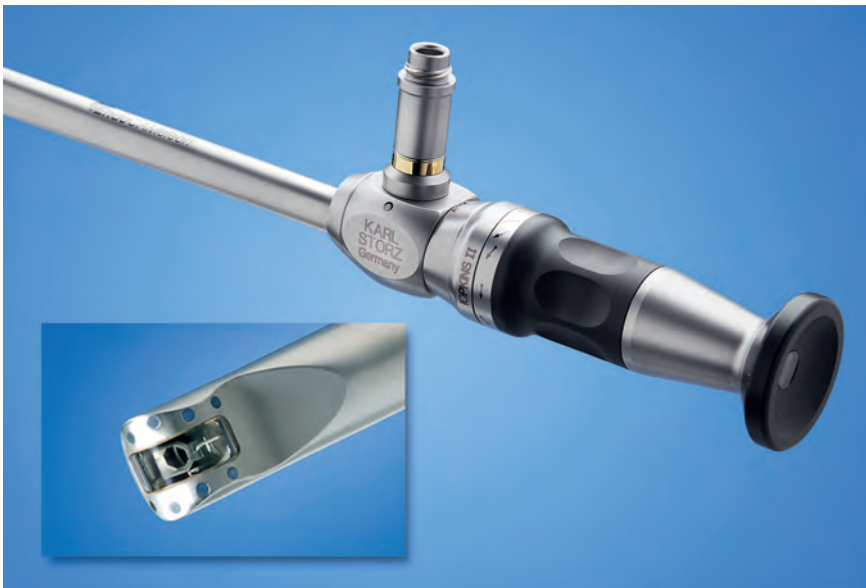
Fig. 2.16 The ENDOCAMELEON ® (KARL STORZ Tuttlingen, Germany) is a versatile laparoscope that allows the surgeon to adjust viewing directions from 0 to 120° as determined by operative circumstances and individual preferences of the surgeon. The core component of its unique design is a swing prism (insert image) at the distal tip of the scope. While image orientation is maintained as in any rigid standard scope, the direction of view is selected by simply turning a rotating wheel until the desired angle is indicated on the dial.
