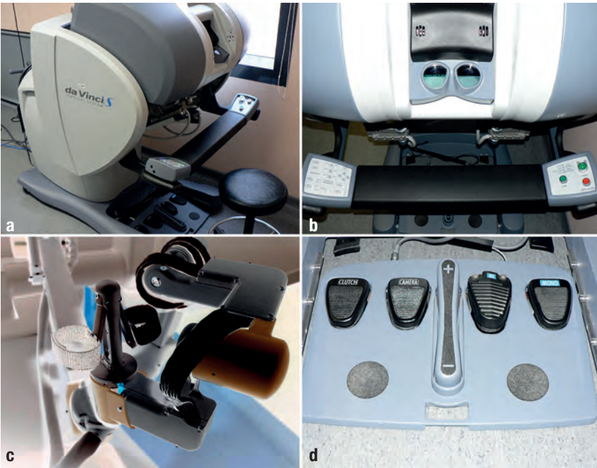
Fig. 4.40 Surgeon console (a, b). The surgeon's fingers grasp the master controls below the display with hands and wrists naturally positioned relative to the eyes (c). Video camera, energy devices, and the 'master controls' can be operated via foot pedals (d).
