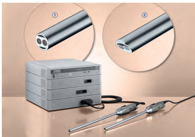
Fig. 2.28 IMAGE1 S camera platform with D3-LINK and TIPCAM®1 S 3D LAP endoscopes. The insert images show the distal end of the TIPCAM®1 S 3D LAP with 0° (1) and 30° (2) direction of view (KARL STORZ Tuttlingen, Germany).
