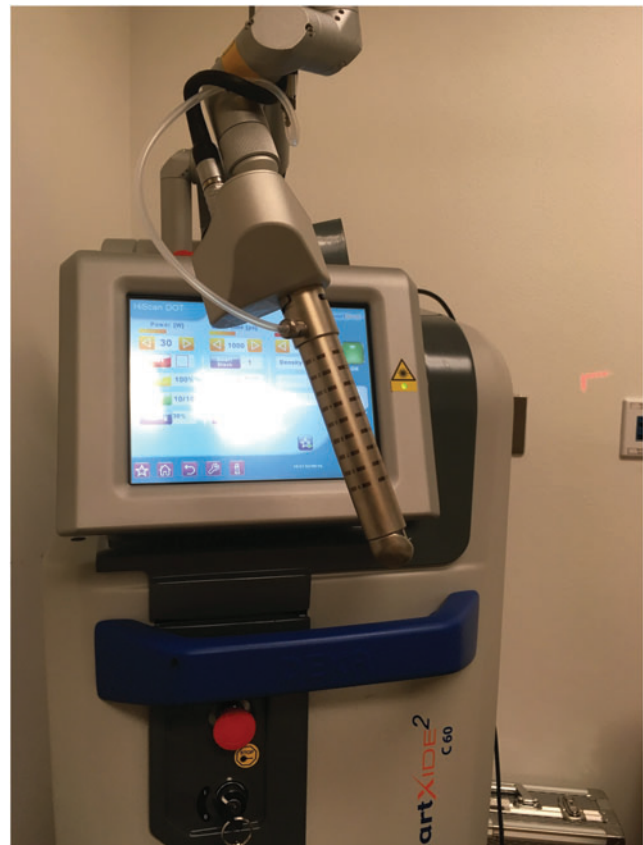
FIG. 1. The Monalisa Touch® SmartXide V2LR CO 2 laser with a vaginal probe attached to an articulated arm.
